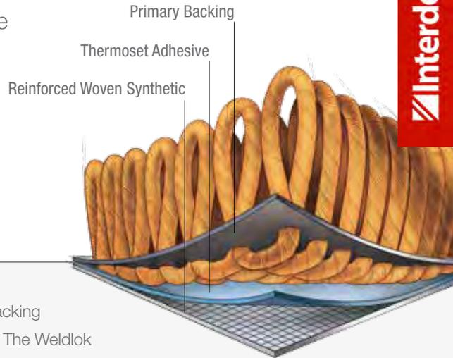
Weldlok® is the Mohawk Group's standard broadloom backing system specifically designed for commercial applications. The Weldlok backing is laminated to our products utilizing a commercial thermoset adhesive. This adhesive is designed to encapsulate and penetrate the carpet back stitch in the main application coat, while the second application coat secures the secondary backing to the carpet substrate for a cost effective performance standard.
